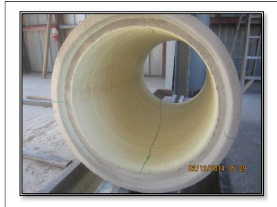
Figure 5- Lined Concrete Pipe at Failure
