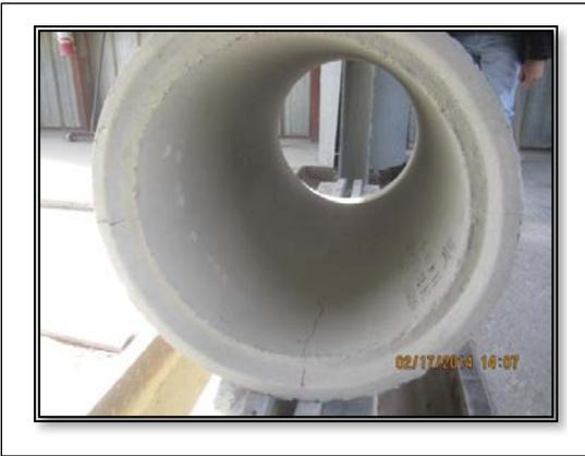
Figure 4- Unlined Concrete Pipe at Failure
