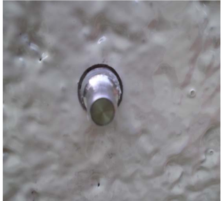
Figure#2: Example of Scored Adhesion Dolly on Coating.
