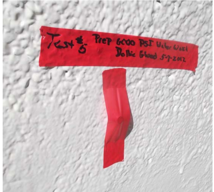
Figure#2: Example of Adhesion Test Dolly Set and Labeled.
