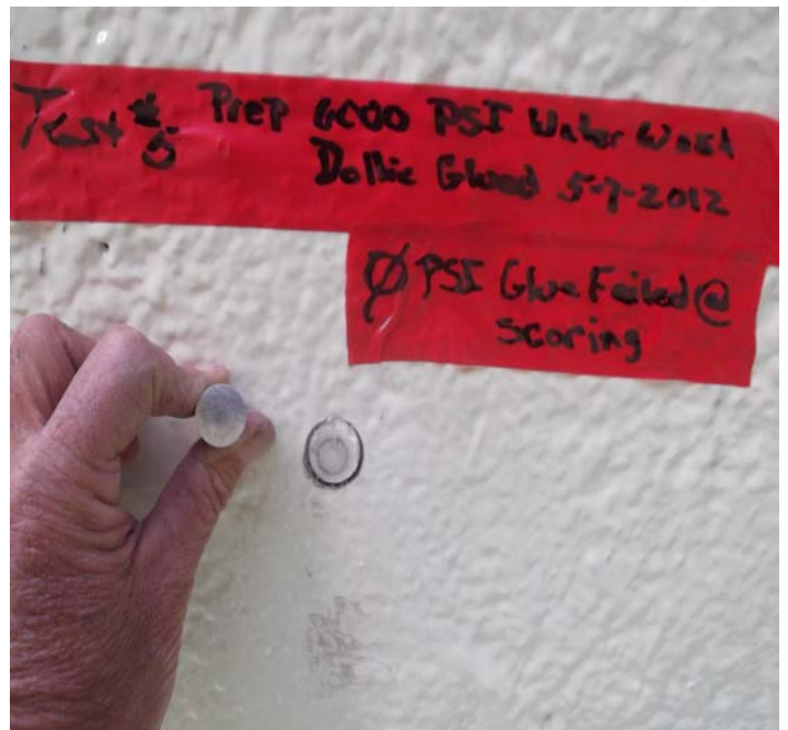
Figure#4: Scored Dolly Failure at Dolly to Glue.
