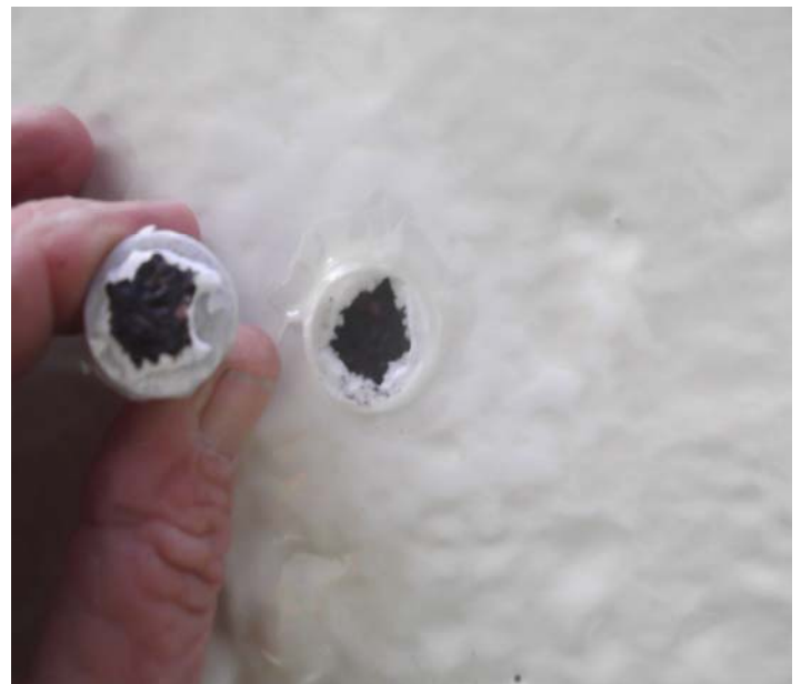
Figure#4: Site #7, No Score 800 PSI Coating Failure.
