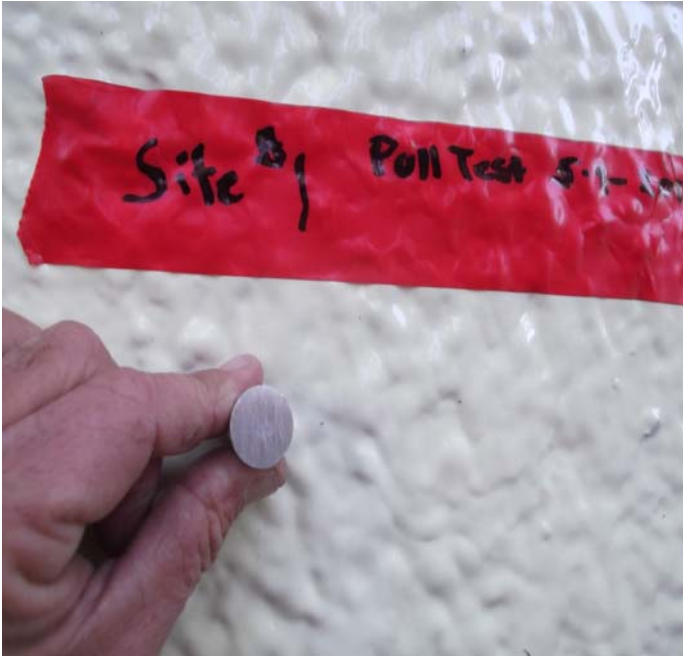
Figure#1: Example of Adhesion Dolly with Incorrect Prep.
