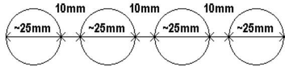
**Figure 1** Layout of the first group of holes on the bare metal pipe.
